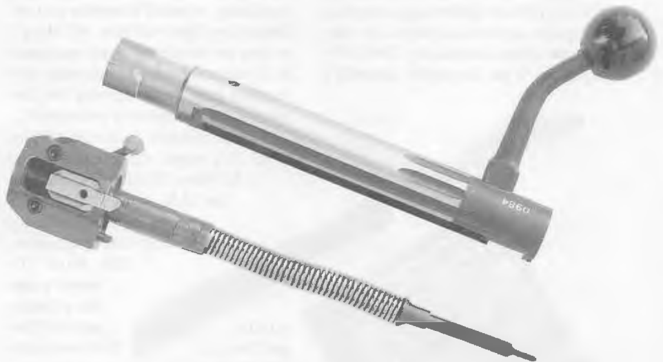
AW/AWP's bolt has three forward lugs. Removal of the cocking piece and spring-loaded firing pin from the bolt body is quite simple. Note lightening grooves on bolt body which also provide an area for the accumulation of debris.
